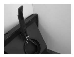
2. Open sealing kit supplied and glue sealing rope into channel on rear edge of appliance. Some types of fire cement/glue are caustic and should not be allowed to come into contact with the skin. In case of contact, wash immediately with plenty of water.
