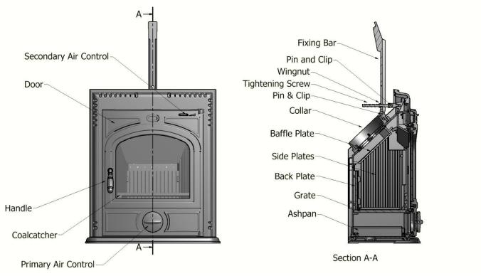
Fig 2 – SR5i Stove Assembly and controls
