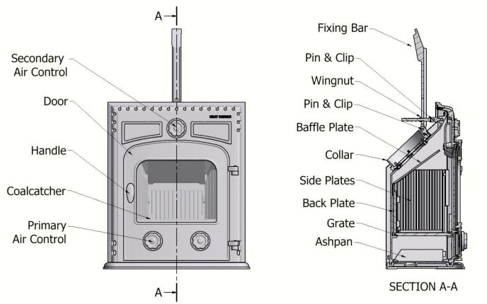
Fig 2 – GR6i Stove Assembly and controls
