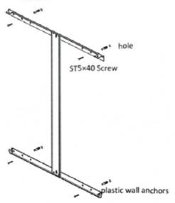
5.6b For 890E and 1500E, mark and drill four holes on the wall using this kind of wall bracket as a template and Fix the wall mount bracket onto the wall with ST5\*40 screws.
