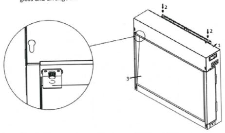
5.6d Secure the front panel onto the appliance by hooking the screws on the panel into the key hole slots on the appliance following the direction as shown.
