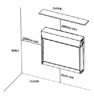
5.6a For 480E and 780E, carefully, mark and drill four holes on the wall using the following wall bracket as a template and push in the four plastic wall anchors. Fix the wall mount bracket onto the wall with four ST5\*40 screws.
