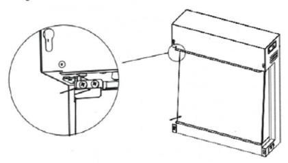
5.5e Position the fuel bed items to your own liking, we suggest you lay a layer of small crystals to cover the fuel bed base then arrange the other items of your choice. Replace the glass panel in revised order of 5.5c and 5.5d for 480E.
