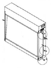
5.4b For 480E, Fix the glass retaining brackets offered as an extra spare part by side and the front.
