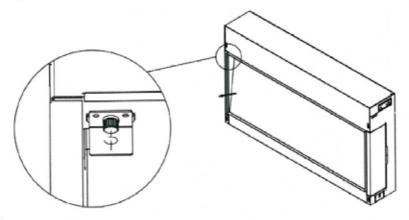
5.5d For 480E, Remove the front glass panels by removing the screws and fixing brackets and then remove the front glass by pulling forward and lifting out of groove.
