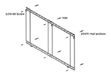
5.6c Put the fire box onto the wall bracket and then fix with two fixing screws of the wall mount brackets on the top of the fire box. Remove the front glass and arrange the fuel bed as described in 5.5d and 5.5e.
