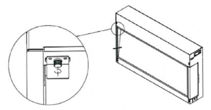
5.5d For 480E, Remove the front glass panels by removing the screws and fixing brackets and then remove the front glass by pulling forward and lifting out of groove.
